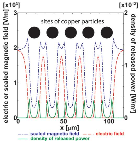
Fig. 6. The amplitudes of the electric and magnetic fields and density of the released energy along the test line shown in Fig. 5. Dashed (red) and dot-dashed (blue) lines represent the electric and magnetic fields, respectively, and the solid line (green) shows the density of released energy. The magnetic field is scaled as  $\eta_0 H$  ( $\eta_0=376.73 \Omega$ ).
