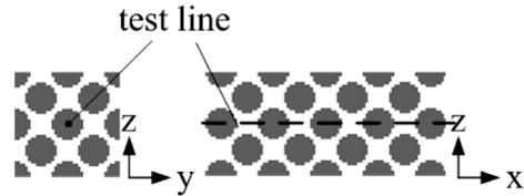
Fig. 5. The configuration of metal particles arranged in body-centered cubic lattice sites. The particle radius is  $R=6 \mu\text{m}$ , the distance between centers of adjacent particles is  $20 \mu\text{m}$ . Data are sampled along the test line.
