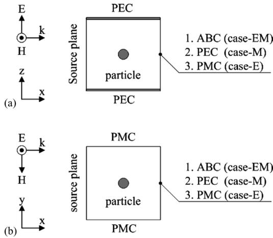
Fig. 1. Scheme of the numerical model. A single metal sphere is placed between the pair of parallel PEC and PMC plates normal to the z and y-axes, respectively; sideview of (a) x-z plane and (b) x-y plane. Microwaves propagate in the x direction.
