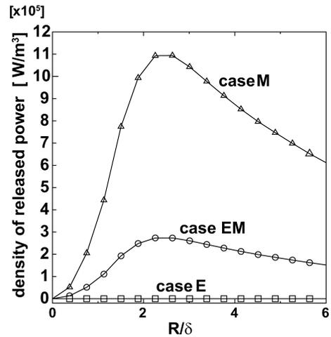
Fig. 2. The density of the released power as the function of the  $R/\delta$  parameter, for three different boundary conditions: case E, case M and case EM., where  $R$  is the particle radius and  $\delta$  is the skin depth.
