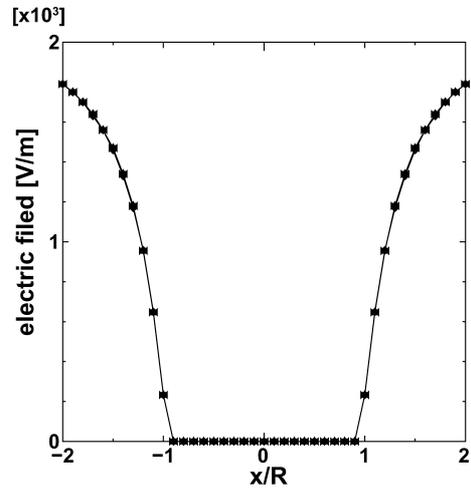
Fig. 3. Distribution of the electric field along the x-axis on the equatorial plane. The origin is set at the particle center. The particle is irradiated by plane traveling waves. The electric field inside the particle is always suppressed. In the shown scale, shape of the electric field distribution does not depend on the particle radius  $R$ .
