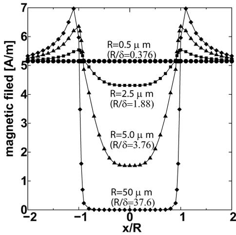
Fig. 4. Distributions of the magnetic field along the  $x$ -axis on the equatorial plane. The origin is set at the particle center. The particle is irradiated by plane traveling waves. Note, when  $R < \delta$  ( $R=0.5 \mu\text{m}$ ), the magnetic field is only slightly disturbed. Here,  $R$  is the particle radius and  $\delta$  is the skin depth.
