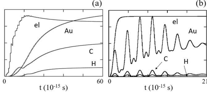
Figure 6: The time changes of kinetic energy of golds, carbons, protons, and electrons for (a)  $5 \times 10^{17} \text{W/cm}^2$ , and (b)  $1 \times 10^{22} \text{W/cm}^2$ . The maximum values are, (a) 0.59 MeV for ions (C,Au,H), and 0.33 MeV for electrons, (b) 42 MeV for golds, and 37 MeV for electrons, respectively. The final value of gold ions is 22 MeV for (b).
