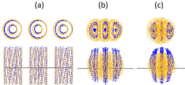
Figure 9: (Color) Merging of a three-array nanotube with double layers inside for (a) 1 fs, (b) 7 fs, and (c) 24 fs, and in carbon (blue) and gold (gold) ions. The scales in the  $yx$ (top) and  $yz$ (bottom) directions are,  $1.3 \times 10^{-6} \text{cm}$ ,  $6.3 \times 10^{-6} \text{cm}$ ,  $2.5 \times 10^{-5} \text{cm}$  for (a) to (c), respectively.
